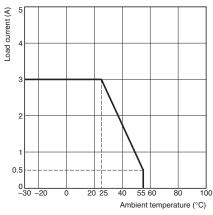
\* When five or more are installed, install with 10 mm space between
