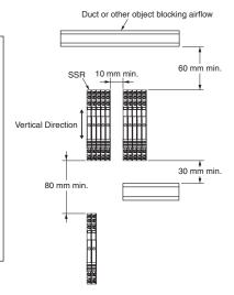
\* When five or more are installed, install with 10 mm space between each.
