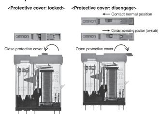
Keep the protective cover open when using the latching lever. Move until the latching lever clicks to the ON position (ON state). After use latching lever, in order to prevent malfunction, return the switch to contact normal position (OFF state), and make sure the protective cover is firmly closed.
